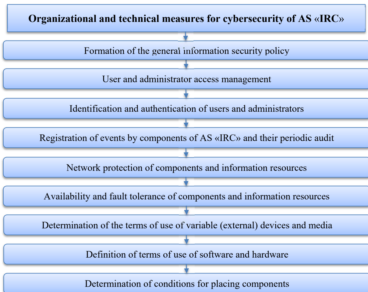
Fig. 2. Organizational and technical measures for cybersecurity of AS «IRC» Compiled by the author based on: [4; 5].
